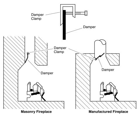
Figure 11 - Attaching Damper Clamp
